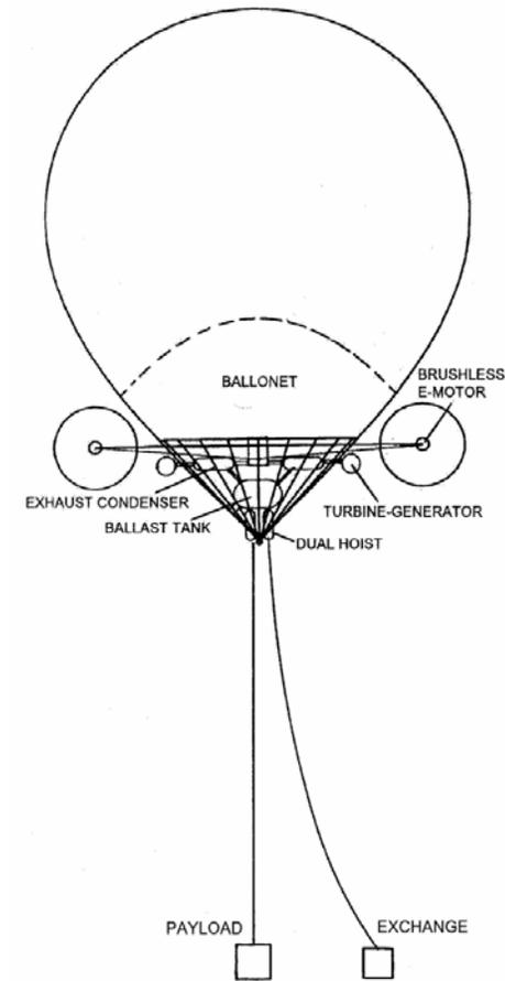
Figure 1 Conceptual Design UAV Logging Airship
