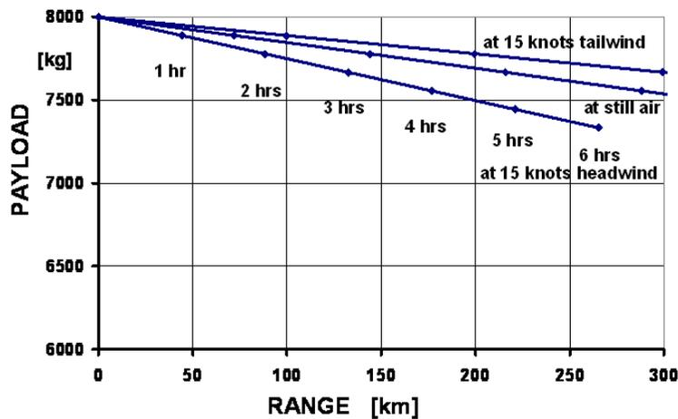
Figure 6 Payload Capacity as a Function of Range and Wind Conditions
