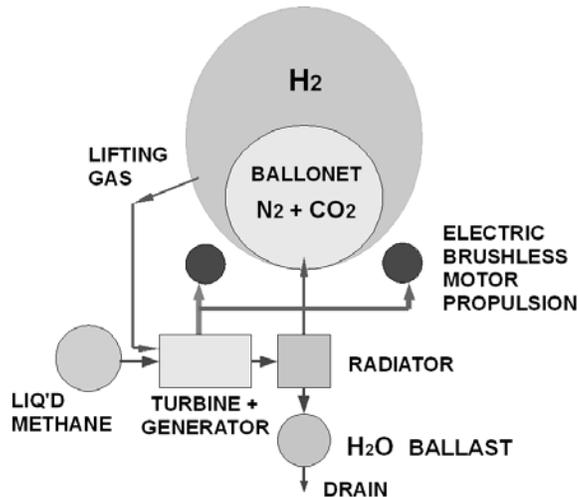
Figure 4: Schematic Overview of the Propulsion Fuel and Ballast System
