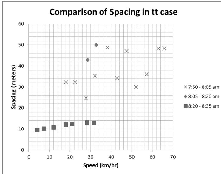
Figure 5 Comparison of Spacing in Truck following Truck
