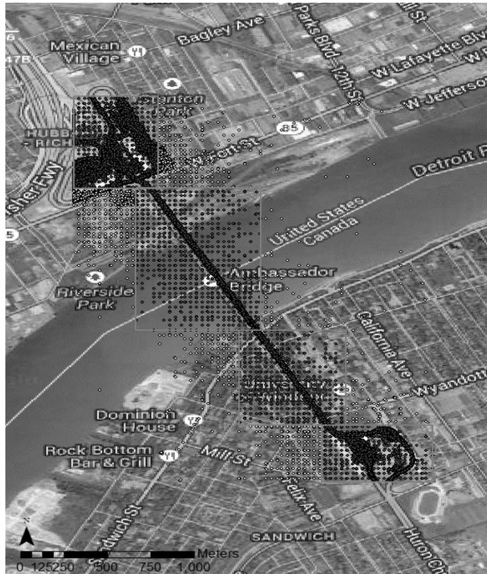
Figure 4. Geo-fence tracking GPS pings of commercial vehicles across the Ambassador Bridge
