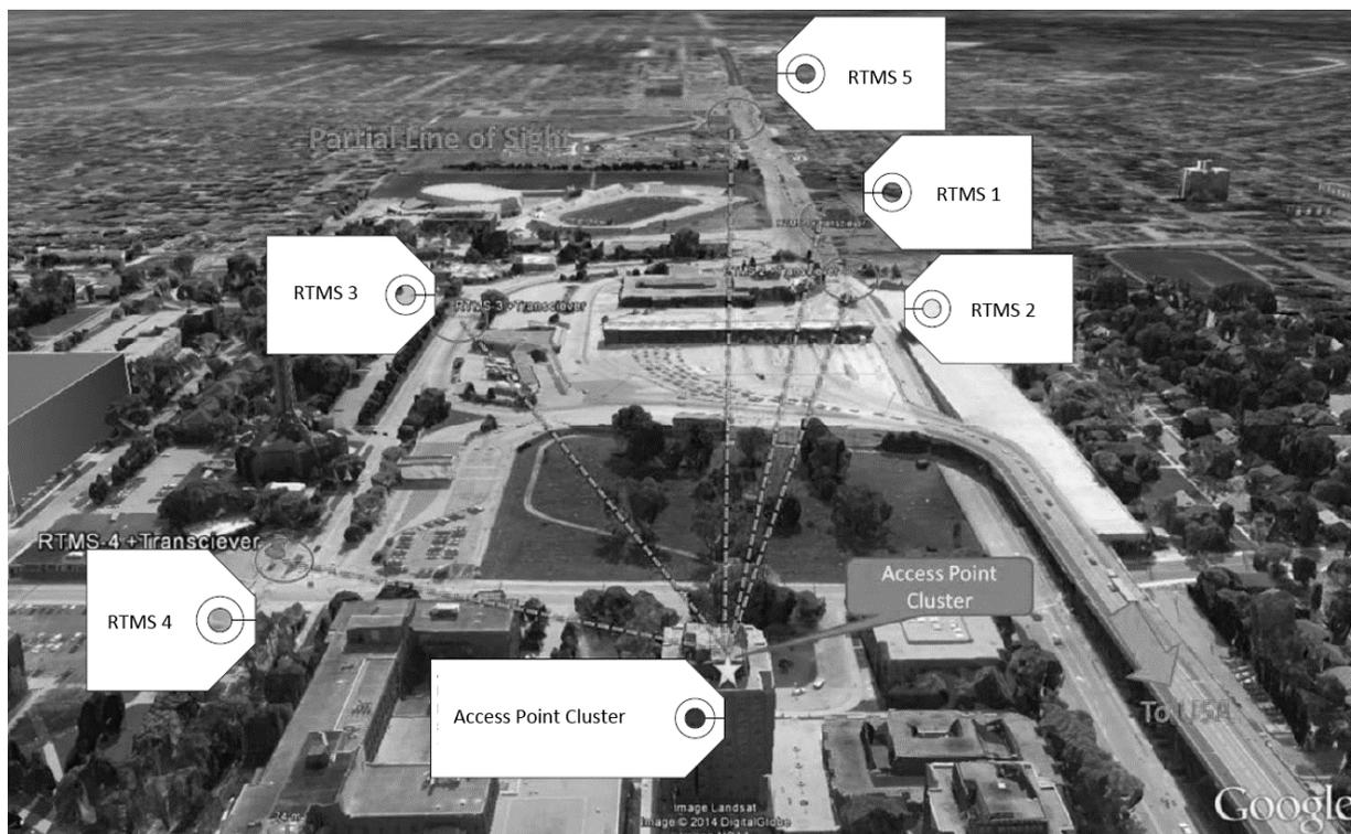
Figure 2. RTMS Data Acquisition System at the Ambassador Bridge (Base Image Source: Google Map)
