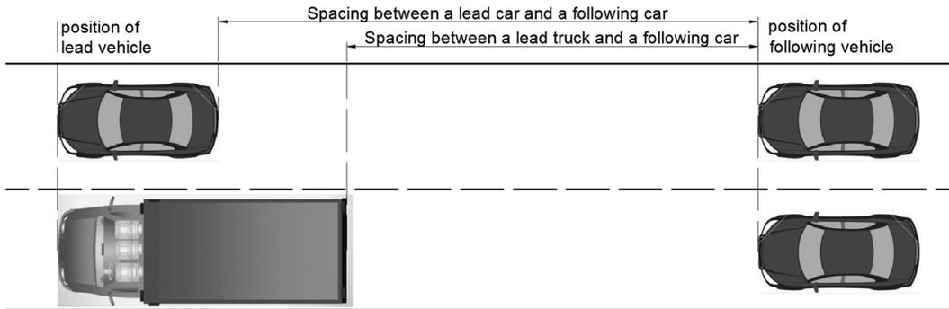
**Figure 2. Comparison of spacing between two vehicles for different length of lead vehicle**
