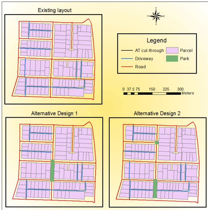
*Figure 1. Fused Grid Design Alternatives*
