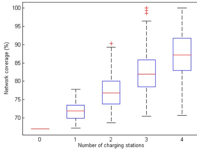
Figure 3- Network coverage for different combinations of charging locations.
