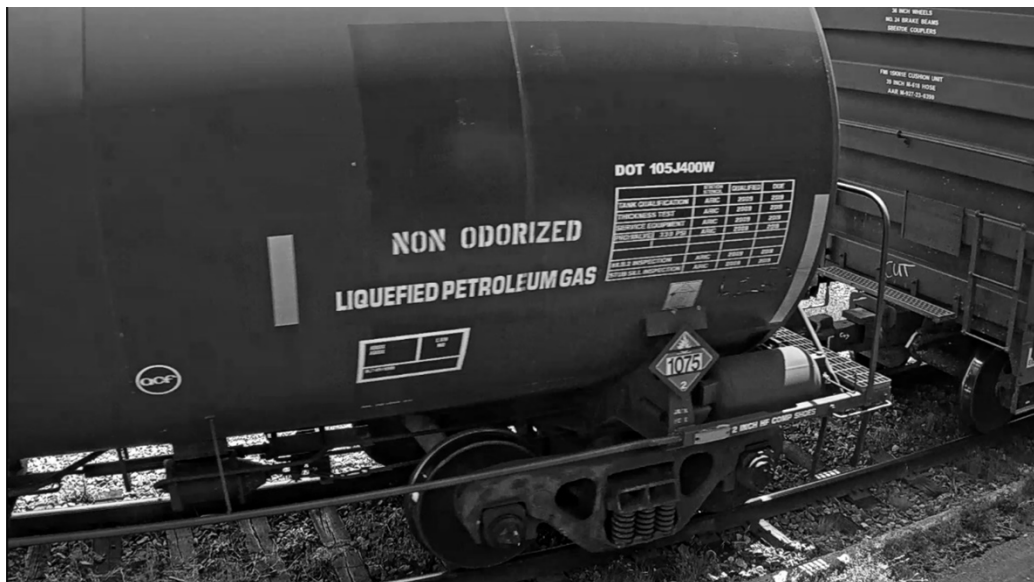
Figure 1 Cargo text, tank car type, and dangerous goods placard legible from the side of passing tank car
