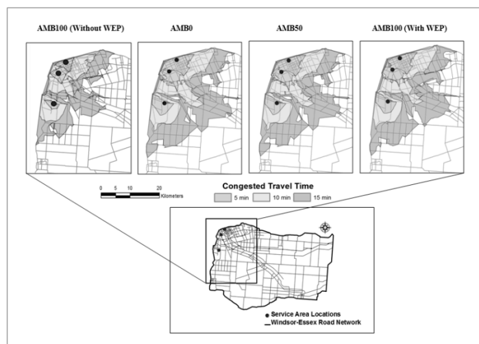
Figure 3. Service Areas under the Base Scenario and the Three Simulated Border Crossing Scenarios for 5, 10 and 15 Minute Drive Times – 4:00 pm
